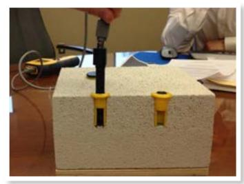
To that end, ASTM F2170-11 recommends the use of in situ probes to obtain accurate relative humidity measurements. This is a big improvement over the calcium chloride testing which is less reliable in that calcium chloride testing only indicates moisture in the top 3mm (1/8"), and are prone to false positives.
