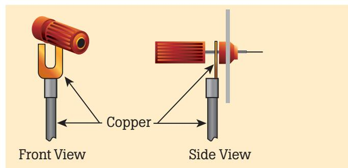
Figure 2: Low resistance connection using a spade lug.
