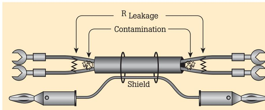
**Figure 5:** Contaminated cable.
